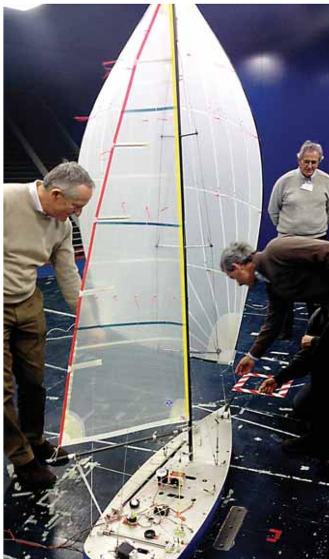
Chair Alessandro Nazareth (left) and other ITC members joined North Sails Italy in a recent continuation of sail tests in the wind tunnel at Milan Polytechnic. The goal is to refine calibration with a parallel study using OpenFOAM software at the Wolfson Unit
