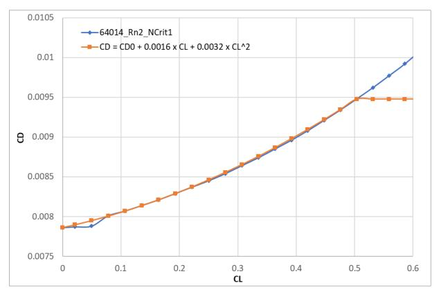
The keel and rudder CL values are to be calculated based on the estimated side force load sharing which changes with the heel angle. The new form factor and CD as a function of CL will be included in 2020 VPP
