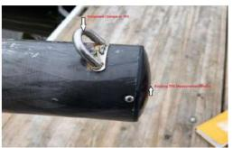
In the case of a J109 (see photo above), the new TPS dimension would be 80 mm shorter and the GPH and APH both increase by 0.2 with the change in TPS measurement. This change will not impact most custom boats such as TP52s which use a "pig nose" trumpet bowsprit tip.
