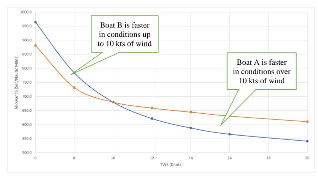
In a typical Performance Curve plot, the vertical axis represents the average speed of the boat around the race course, expressed in seconds per mile. The horizontal axis represents the wind speed in knots. When the finishing time of a boat is known, its elapsed time is divided by the distance of the course to determine the average speed in seconds per mile.
