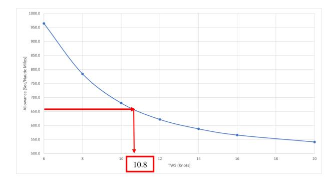
The corresponding point on this curve on the horizontal axis is the so-called Scoring Wind. This means the yacht has completed the course "as if" it has encountered that wind speed. The faster the boat has sailed, the higher the Scoring Wind, which is the primary index used for Polar Curve Scoring: the yacht with the highest Scoring Wind wins the race.
