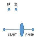
From the course constructed as described above, the true wind angle (TWA) is calculated as being the difference between the wind direction and compass bearing of each leg. With this information, a table is made for each boat that describes the theoretical speed of that boat over that course for the range of seven true wind speeds (TWS). Calculated time allowances for these wind speeds are then used to calculate Scoring Wind and corrected times as explained above.
