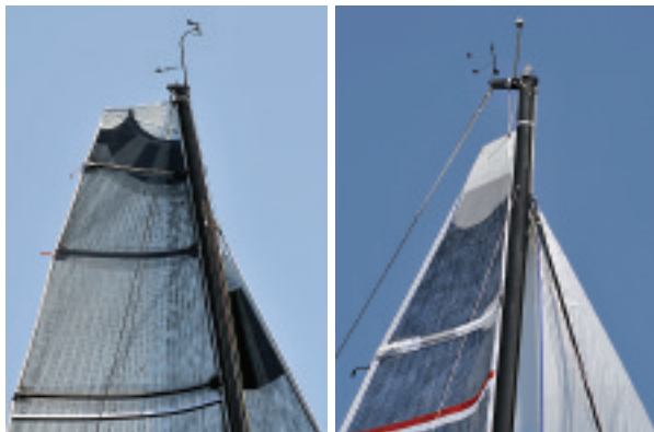
Top: fast in ORC in 2010, the Grand Soleil 42R Man which won the European title in Cagliari is a 2005 Botin & Carkeek IMS design. If there was not so much carbon involved the GS42R would make a good IRC racer... albeit with the bulb keel option. A contrast in IRC (left) versus ORC (right) headboard treatments – there is no IRC headboard measurement allowing a modern square profile but requiring a backstay flipper or a pair of running backstays
